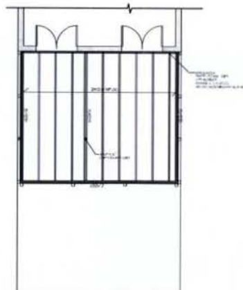
3 DECK FRAMING PLAN 1/4" = 1'-0"
