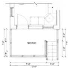
1 DECK FLOOR PLAN A1 SCALE 1/8" = 1'-0"
