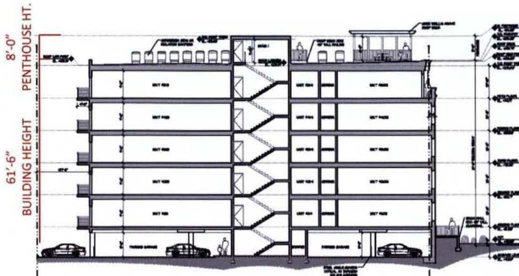
1 BUILDING SECTION A3-0 SCALE: 1/20" = 1'-0"
