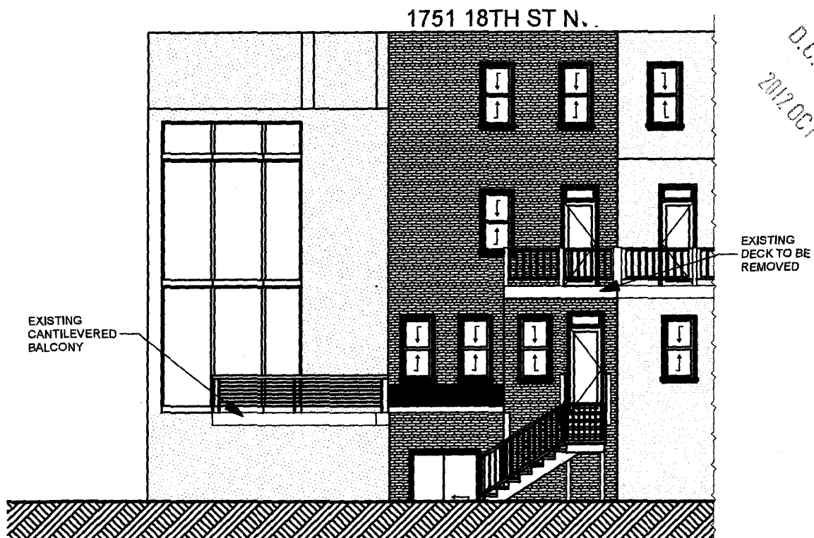
EXISTING REAR ELEVATION
