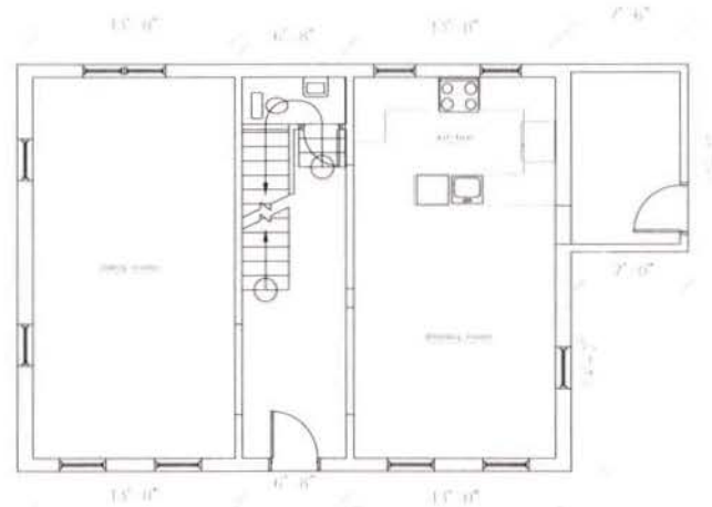
FIRST FLOOR PLAN SCALE: 1/4"=1'-0" 980 sq ft
