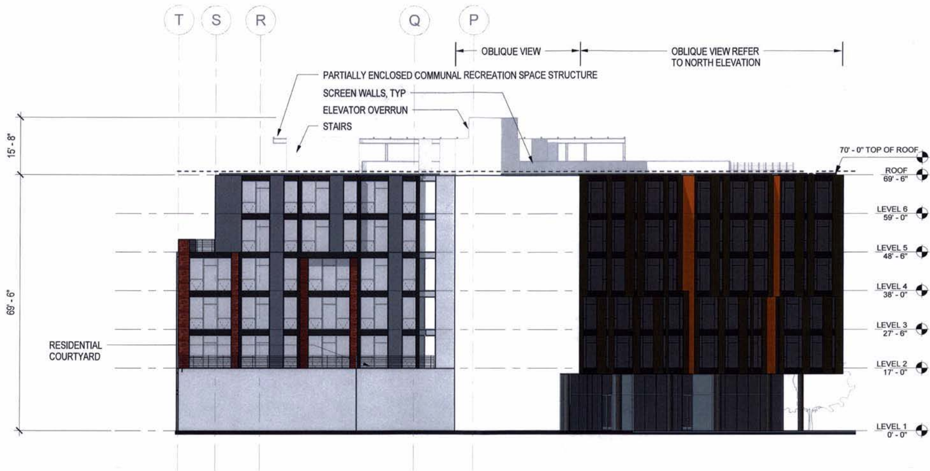
1 EAST ELEVATION - EAST BLDG 1/16" = 1'-0"
