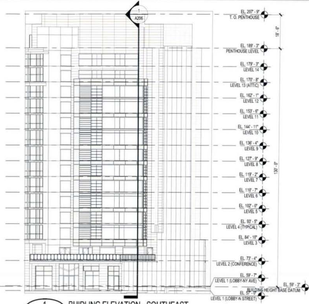
1 A204 BUILDING ELEVATION - SOUTHEAST SCALE: 1" = 20'-0"
