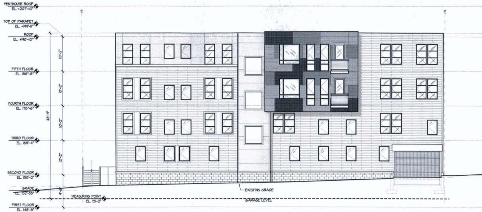
A4.2 EAST ELEVATION (ALLEY) SCALE: SCALE 5/32" = 1'-0"
