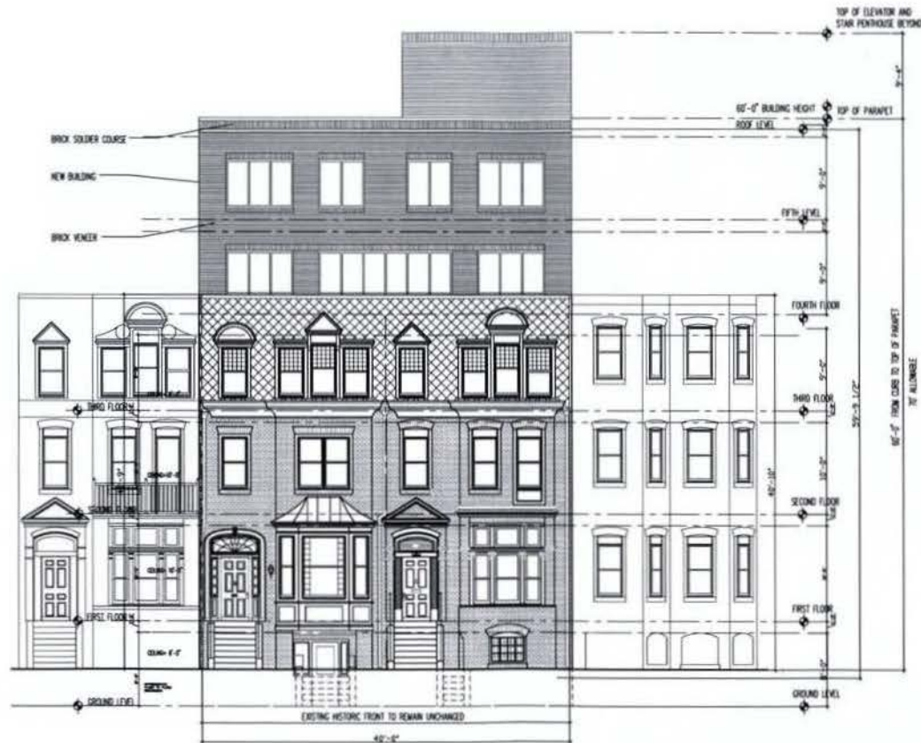
FRONT ELEVATION ON JEFFERSON STREET SCALE: 3/16"=1'
