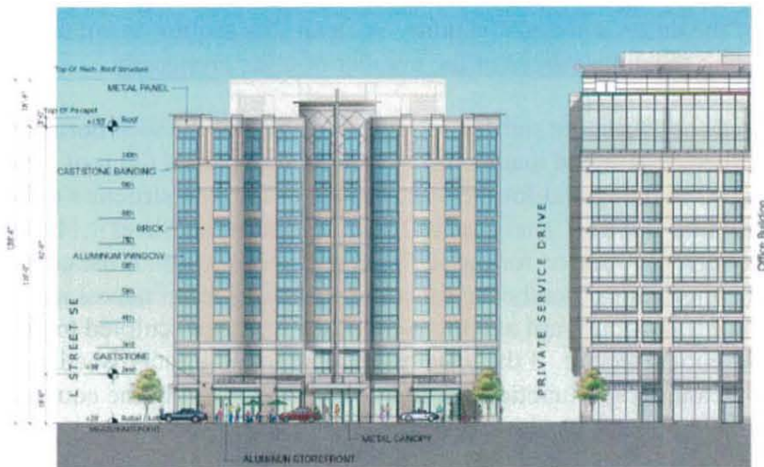
Figure 5: Revised Façade of Square 769 Proposed Apartment Building
